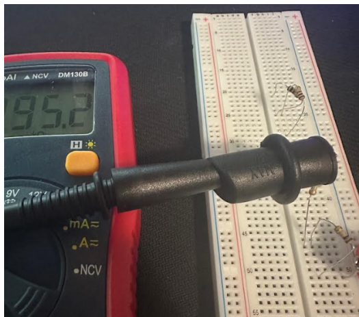
Figure 1.1.1: Showcases the circuit with 2 100k ohm resistors in series.
