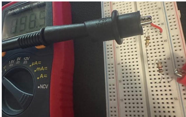
Figure 1.1.1: Showcases the circuit with 2 100k ohm resistors in series.
