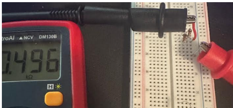
Figure 1.1.3: Showcases the circuit with a 1k and a 100k resistor in parallel.
