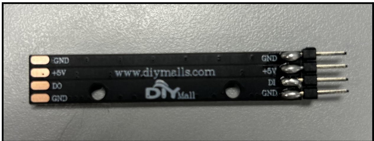
Figure shows one of the LED strips with the right side soldered and the left side unsoldered.
